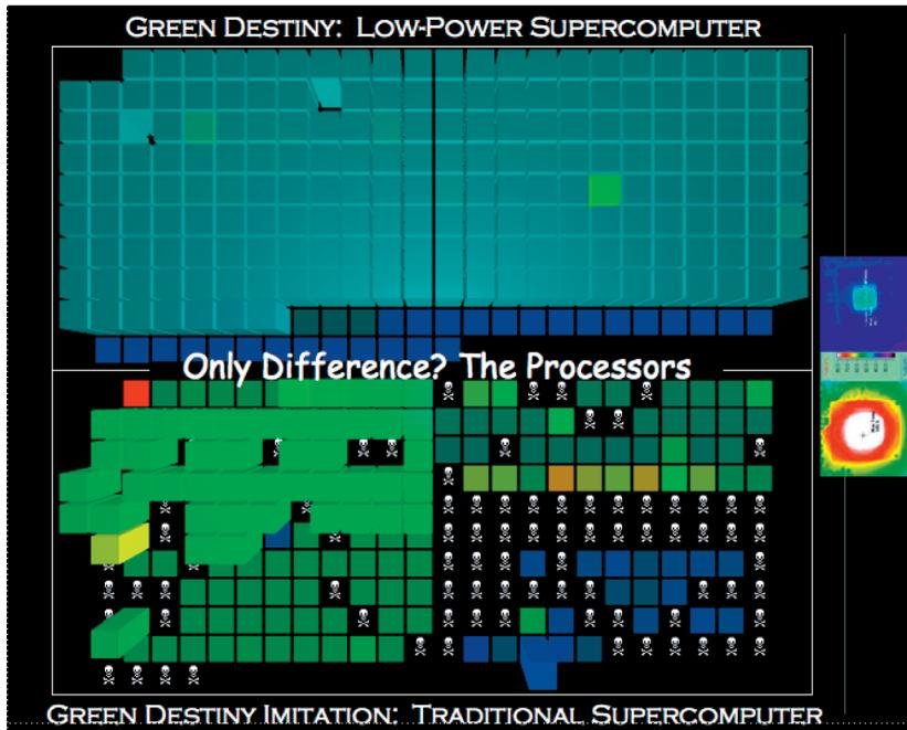
**1 Green Destiny's reliability versus its imitation. Both systems have the same number of nodes, as represented by each square-shaped area, and run the same applications without any special cooling facilities. The only difference is that Green Destiny uses ultra low-power processors whereas the imitation uses higher-powered "low-power" processors. Green Destiny has no failed nodes, whereas more than one-third of the traditional imitation nodes are dead (shown with skull and crossbones).**
