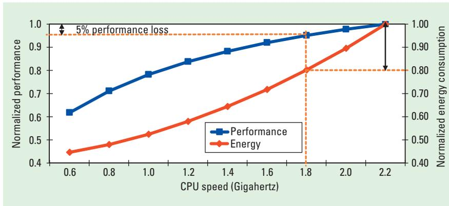
**2 Energy–performance trade-off.** For certain workloads, we can scale down the processor to save 20 percent in energy costs while losing only 5 percent in performance. This 5 percent loss means that an application that normally takes 57 minutes to run would take one hour but would have a 20 percent reduction in energy consumption, which translates to \$2 million in energy savings.
